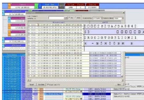
Figure 12 Hard drive S/N as displayed on the SATA Sierra M6-1 SATA protocol system
